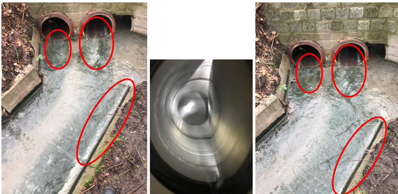
These pictures show the entrance to the trench at the beginning of the experiment on the left and a day later on the right. It can be seen that the deposits have decreased significantly, which I could also be seen in the pipeline to the boiler housing from drying 2. There has always been a very light, slimy coating, which is no longer present a day later, or has rebuilt.
