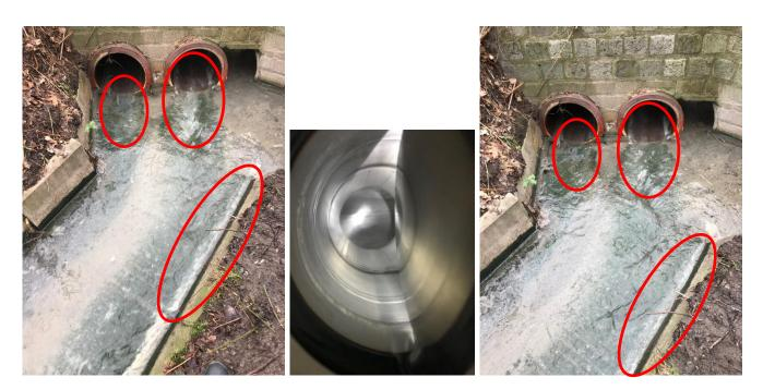
These pictures show the entrance to the trench at the beginning of the experiment on the left and a day later on the right. It can be seen that the deposits have decreased significantly, which I could also be seen in the pipeline to the boiler housing from drying 2. There has always been a very light, slimy coating, which is no longer present a day later, or has rebuilt.
